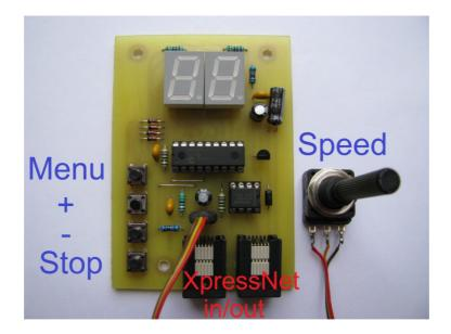
Locomotive address. When you connect Mouse that shows the last used locomotive address. Press "+" button to change direction. Press button "-" to on/off locomotive light (function F0).
